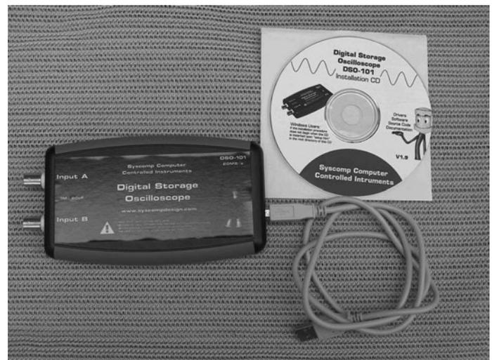
Figure 1 DSO-101 hardware and application software
