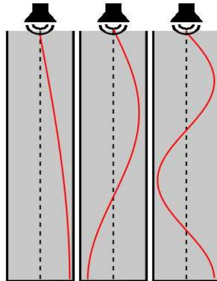
Figure 2: Pressure Distribution in a Closed Tube:
