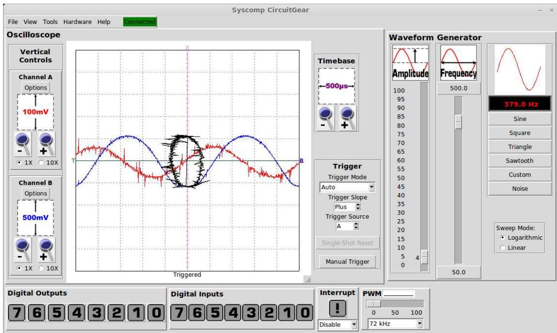
Figure 6: CGR-101 Screen Shot: Resonance Display
