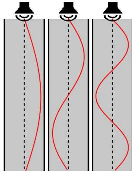
Figure 1: Pressure Distribution in an Open Tube:
