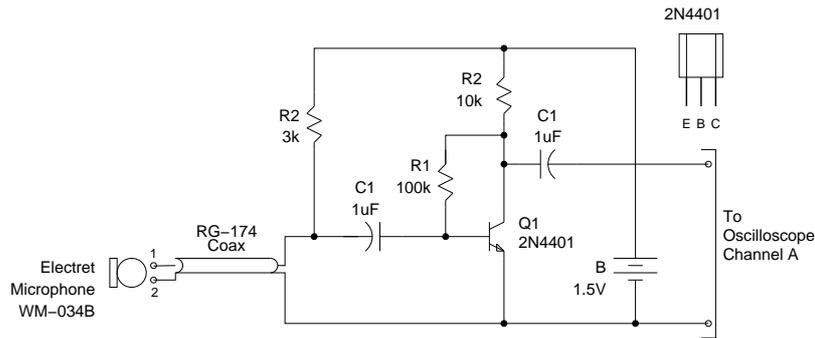
Figure 4: Microphone and Amplifier
