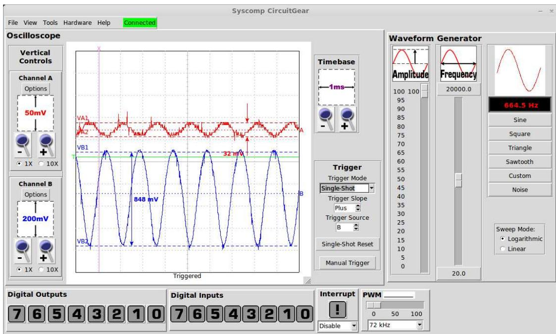
Figure 5: CGR-101 Screen Shot: Amplifier Waveforms: Channel A, Input. Channel B, Output
