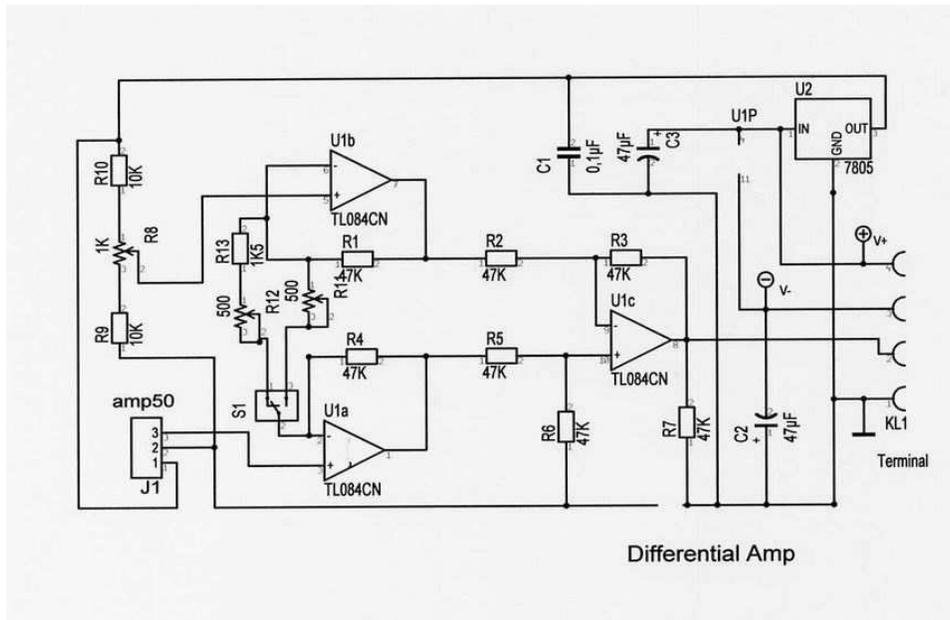
Figure 7: Hall Effect Sensor, Differential Amplifier Schematic
