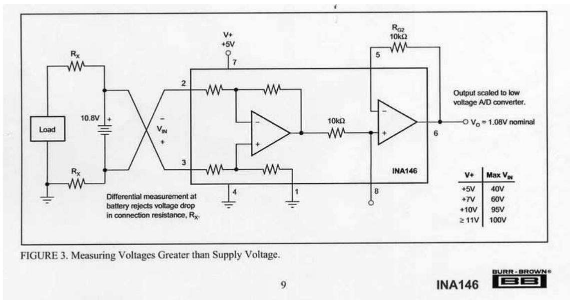
Figure 4: Differential Amplifier Schematic
