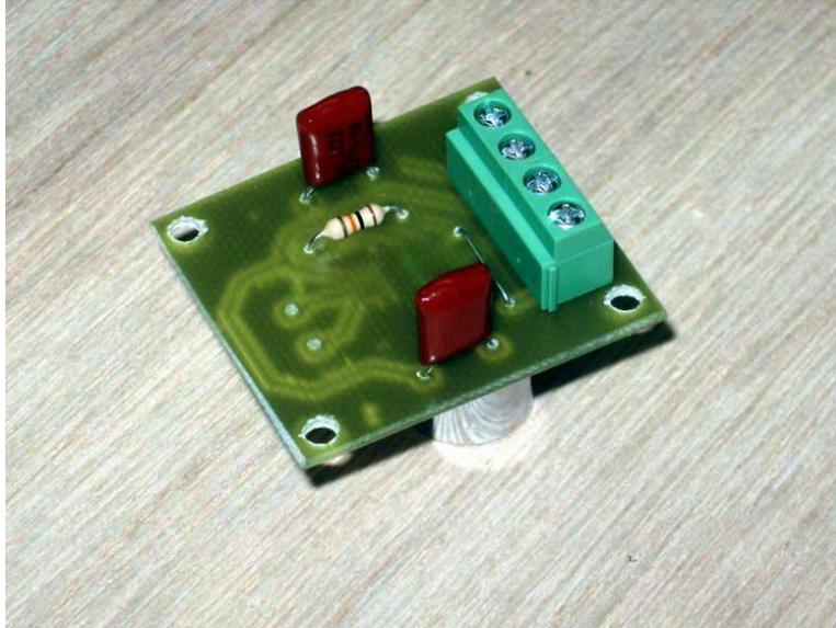
Figure 5: Differential Amplifier Assembly
