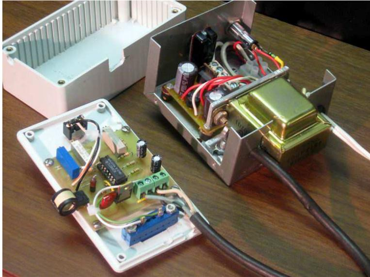
Figure 8: Hall Effect Sensor Assembly and Power Supply. Notice the Hall Effect Sensor on the amplifier circuit board, left side.
