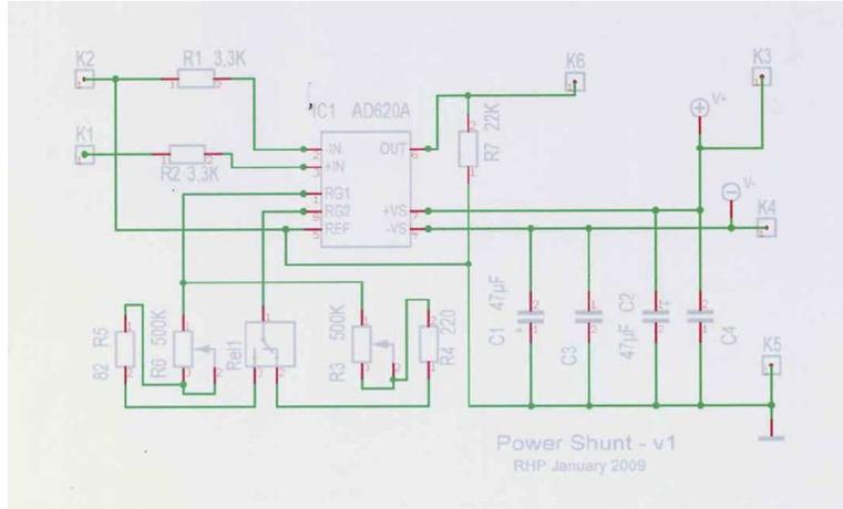
Figure 2: Powered Shunt Schematic
