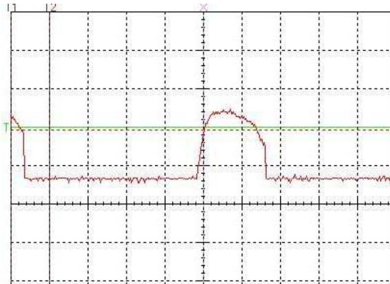
Figure 9: Current Waveform (1 amp per vertical division)
