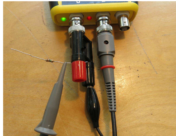
Figure 5: \times 10 Probe Loading Circuit
